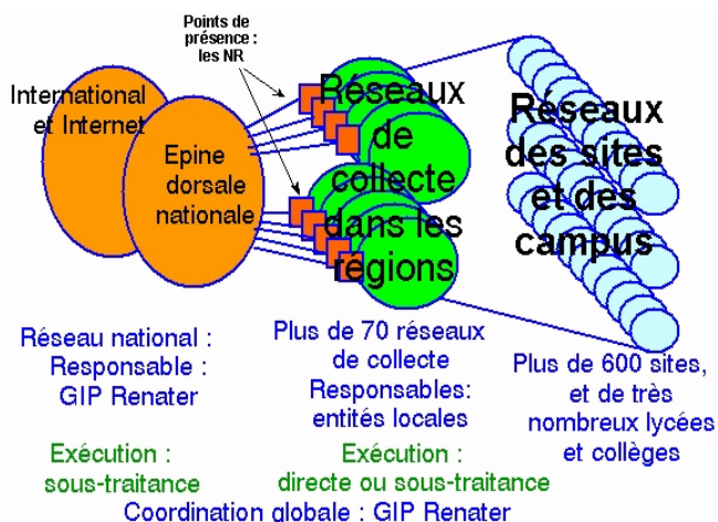
Figure 1 : Principe de structuration de RENATER (source Renater)
